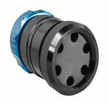
**Spider Clamp-** The P3-19 pin Spider Clamp offers cable strain relief combined with watertight sealing when using 6 individual cables in breakout applications. The design incorporates our "Spider Trap" mechanical grip mechanism which individually grips each cable jacket. The trap can be quickly and easily orientated to facilitate different cable diameters. A separate silicone grommet ensures a watertight assembly.
