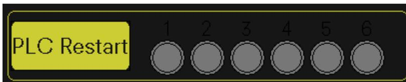
The PLC Restart section has indicators for each PLC’s encoder counters. They all must be green for the system to run. If they are not green press the “PLC Restart” button. This will re-initialize the counters.
