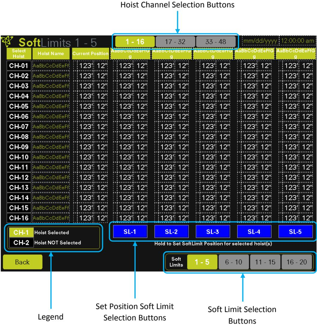
**Hoist Channel Selection Buttons** - All 80 hoist’s information cannot fit on one page. Use these buttons to choose the set of 16 hoists you wish to modify.
