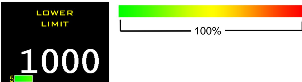
The 10 segment bar graph display is multicolor in order to provide you with a visual telltale of the measured weight. The weight readout numerals will turn red once you have reached a 120% overload threshold. Additionally, this activates a SPDT relay with normally open and normally closed contacts. This can be used as a safety shutdown, to operate an external audible or visual alarm or any other user defined application.
