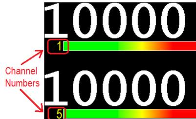
Each of the 8 weight readout displays have a user settable number. If your setup has more than one **Cell\*Mate Display** you can assign a number to any channel you wish from 1 to 999. This number is only a numeric label and does not affect the Cell\*Mate system in any way.
