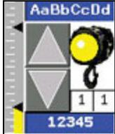
Shows motor status as 'Under Weight (Slack Chain)'. The bar graph will be yellow in color and the motor status icon will be yellow and blinking. Once any channel that has reported an underweight (slack chain) fault, it will ONLY be allowed to move in the up position.
