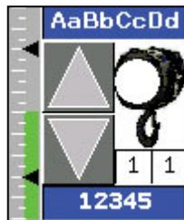
Here is a breakdown of the above image. You will notice the bar graph on the left that indicates the amount of weight on that particular Load Cell. In that bar graph you will notice two black triangles. They represent your upper and lower limits. The bar graph starts at zero pounds and maxes out at 125% of your upper limit.
