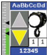
'Down' arrow shown in yellow indicates motor is ready for movement in the 'Down' direction.
