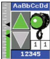
Motor status Icon and 'Up' arrow shown in green indicates motor is moving in the 'Up' direction.
