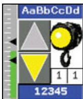
Motor status Icon and 'Down' arrow shown in yellow indicates motor is moving in the 'Down' direction.
