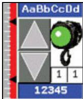
Shows motor status as 'Over Weight'. The bar graph will be red in color and the motor status icon will be green and blinking. Once any channel that has reported an overweight fault, it will ONLY be allowed to move in the down position.
