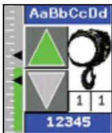
'Up' arrow shown in green indicates motor is ready for movement in the 'Up' direction.
