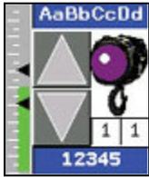
Motor status Icon shown in purple indicates that the Load Cell is NOT plugged into the Cell\*Mate Hub or the data cable from the Load Cell to the Cell\*Mate Hub is damaged.
