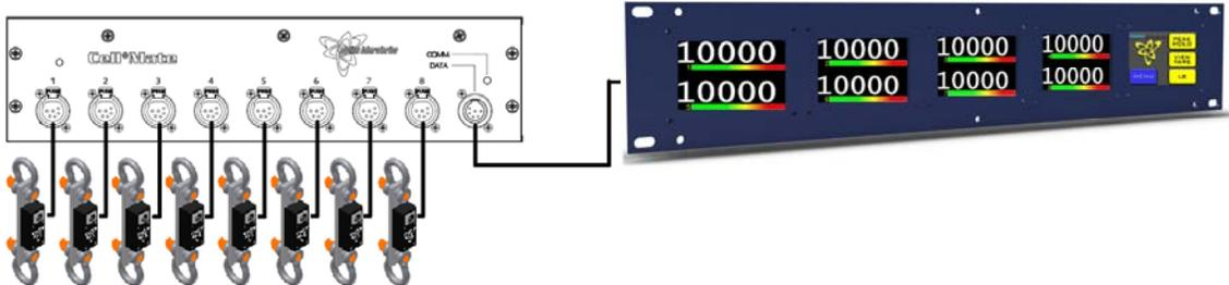
8-channel system setup with more than one display. Note termination switch turned on only on the last display in the chain.
