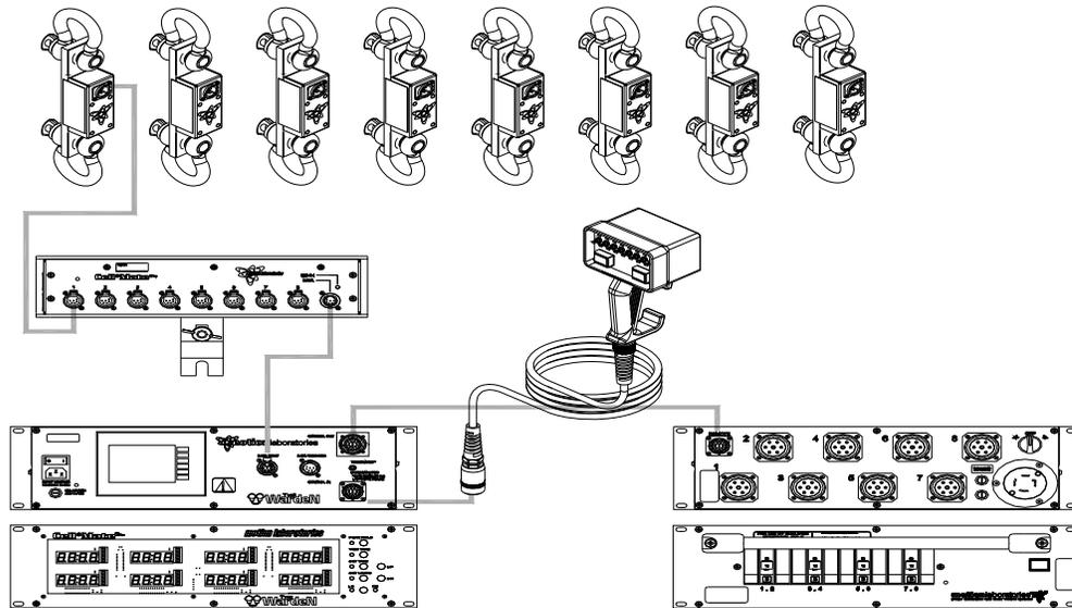
Figure 2 Shows a Cell\*Mate System using the The Warden to oversee a Chain Hoist Control System. For the purpose of clarity we have only shown the first connected Load Cell. Run the data cable(s) and connect each Load Cell to its assigned channel connector on the Cell\*Mate Hub. Connect the data cable from the Cell\*Mate Hub to The Warden. Connect a standard MLI Remote Hand Held Station to The Warden. Connect The Warden to a MLI Chain Hoist Controller using a standard P26 Remote Cable.
