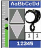
Motor status icon shown in white indicates motor ready to be selected for movement in either direction.
