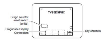
The SPD Diagnostic display shows the status of each IMA module with diagnostically controlled green/red LEDs. If a unit is operating correctly, all of the phase LEDs will be illuminated green. To test the integrity of the diagnostics for each phase, push the button below the phase LED on the display. The green LED will turn red and the alarm will sound (if enabled) Releasing the test button will complete the test; the red LED will turn green and the alarm will shut off.
