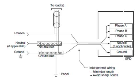
An overcurrent protective device has been installed upstream of the SPD to provide a means of disconnect. Please reference power distribution system wiring schematics for details.
