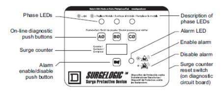
Audible Alarm. Push the alarm enable/disable button to enable or disable the alarm. If the green alarm LED is lit the alarm is enabled. If the green alarm is not lit the alarm is disabled.
