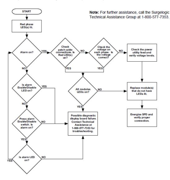
When power is applied to the SPD and one or more of the diagnostic display LEDs are red, and one or more IMA module LEDs are out, the appropriate MA module should be replaced.
