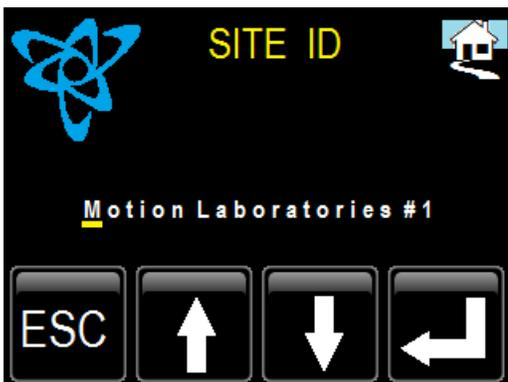
From the main set up page press the “NETWORK” button, then the “SITE ID” button to access this window. To change Site ID use the UP and DOWN arrows to select upper and lower case letters, numbers and standard characters as desired. Press and hold arrow keys for fast scroll through characters. Press the enter key to advance to the next position indicated by the yellow underscore. Up to 22 characters may be used including spaces.
