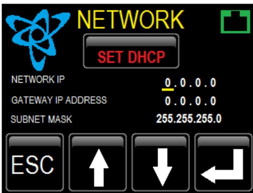
From the main set up page press the “NETWORK” button, then the “SET IP” button to access this window. The network setup page has the choice of changing IP settings for a fixed address or choosing DHCP for automatic addressing.
