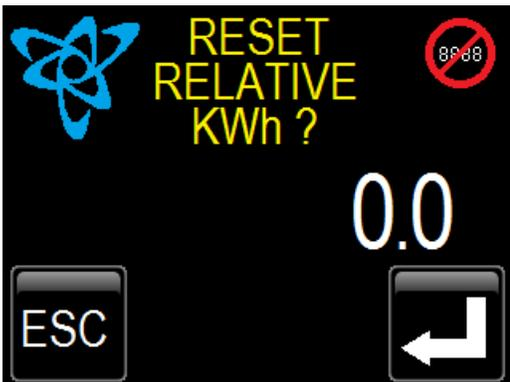
From the main set up page, press the “KWh RESET” button to access this window. When the display is in Power Mode, Kilowatt hours and relative kilowatt hours are displayed. While kilowatt hours is not changeable, relative kilowatt hours can be reset to zero. The display will show present relative KWh. If you escape no change will be made. Pressing the enter key will zero the relative KWh as indicated on the display.
