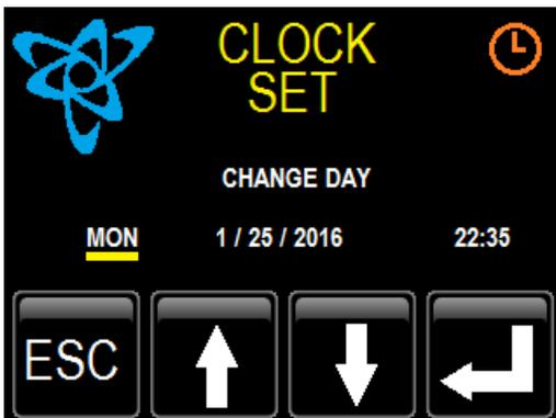
From the main set up page, press “CLOCK SET” to access this screen.
