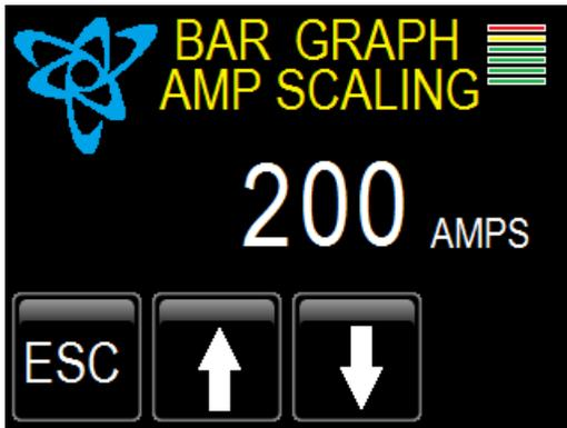
From the main set up page, press the “BAR GRAPH” button to access this window. Bar graph amp scaling allows you to set the range of the 20 segment current bar graph for the X, Y, Z and Neutral displays in the volt amp frequency mode. Use the up/down buttons to adjust the value from 20 to 1000 amps. The bar graph will display all 20 bars when measured current is the same as set current value. Press escape to return to the main setup menu.
