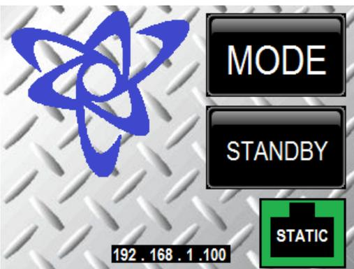
Control screen showing Ethernet connected in static mode with address
