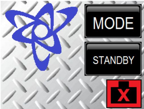
Control screen showing Ethernet disconnected
