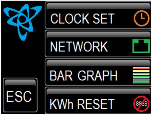
Pressing escape while on the setup menu page will bring you back to the default mode (voltage current frequency mode). When in any setup menu if there are no button presses within 60 seconds the meter will change back to default mode.
