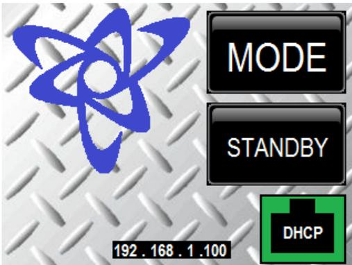
Control Screen showing Ethernet connected in DHCP mode with address
