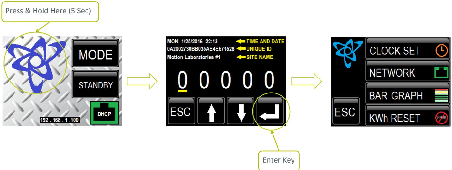
Enter setup mode by pressing the blue Motion Labs logo five seconds. A code entry screen will be displayed. Without entering the code you will be able to see the current time and date of the real time clock and the meter's 24 character unique ID number and the site ID. The unique ID number is required for setup of subscription based remote access website.
