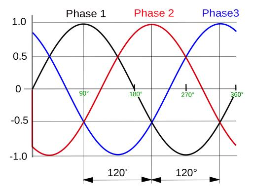
A transformer that is fed, on the primary windings, by three equal alternating voltages, the timing of which are 120 degrees "out of phase" with each other. A typical application would be 480V input with 120/208V output, where the grounded conductor (neutral) on the 120V output is common with all three lines (Phases).
