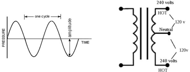
A transformer that is fed, on the primary winding, by a single alternating voltage, which can be represented by a single sine wave. The secondary winding can be "split" or "tapped", to produce multiple voltages, such as, 120/240V.
